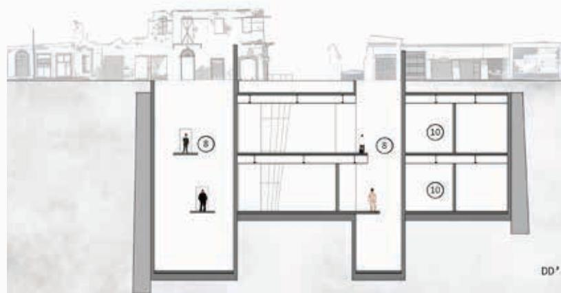
**[Figure 13]** Section DD. The section that includes the frontier wall that is 18 meters high.
